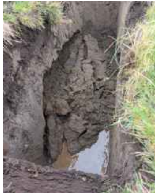
Figure 21A & 21B – Sidewalls in trial pits located in Area 3. Fig 21A Sidewall in TP20 showing firm and firm to stiff clayey SILT and silty CLAY to 2.60m. A firm occasionally soft to firm blackish grey clayey SILT was logged from 2.60m to 3.0m (76.78m OD) Fig 21B Sidewall collapse in BRE SA05. Water sitting at 1.70m bgl.
